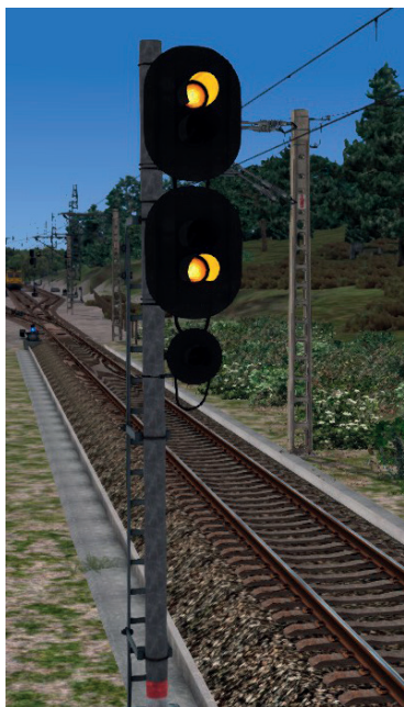
DOUBLE YELLOW: Proceed via diverging points into the station.
