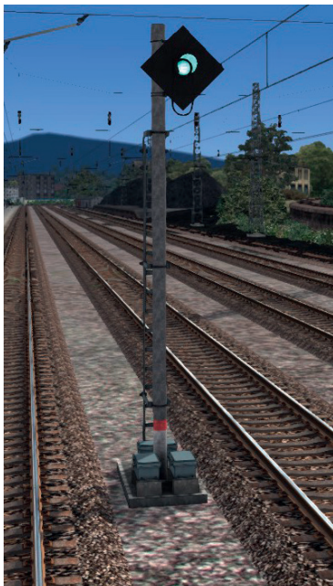
GREEN: This is a Departure Repeat Signal, and the Departure Signal is open (green or yellow).
