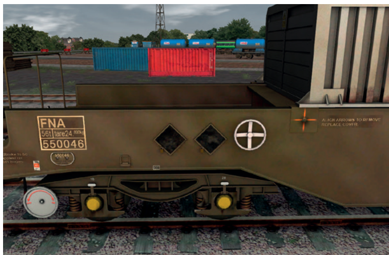
FNA unloaded (no hazard diamonds)
