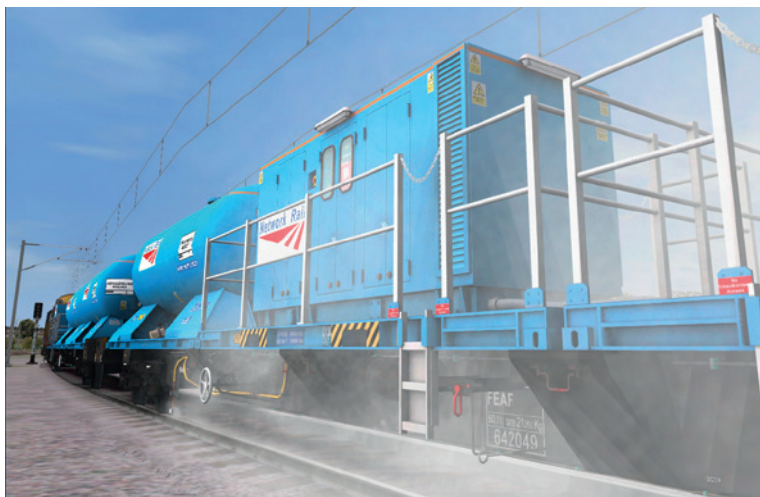
RHTT high pressure water spraying
