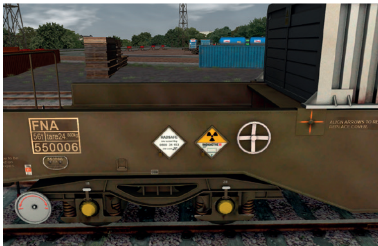
FNA loaded (hazard diamonds visible)
