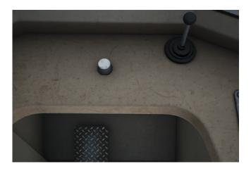
AWS alarm acknowledgement button - press to acknowledge the AWS alarm.
