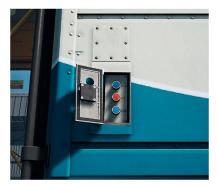
Inside the panel you will see three buttons. Press the red OPEN one to open the doors.
