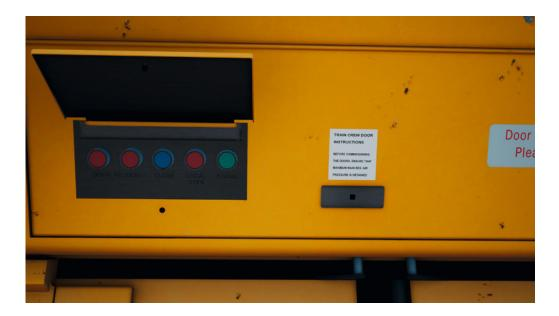
To only open the door which you are standing next to, press the red LOCAL OPEN button. All the other doors will stay closed and locked. If you want to open ALL the doors on the platform side, press the two red DOOR RELEASE buttons.
