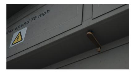
Rotate this handle to change the destination names in the exterior panel.
