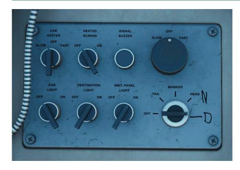
CAB HEATER - move the switch as required (SLOW/OFF/FAST).
