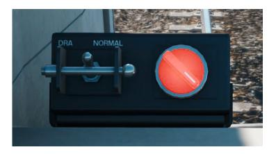
This system is designed to be a defence against SPADs (Signal Passed At Danger). The driver must activate the system when stopped at a station when an adverse signal is displaying. When the system is activated, as shown by the red light being illuminated, the engine throttle is deactivated and therefore the train cannot be driven. Deactivating the system turns off the red light, the throttle is reconnected, and you can drive the train as normal.
