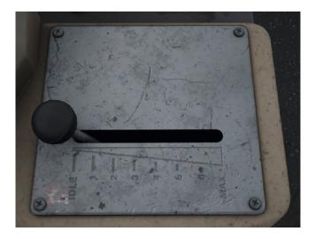
Moving the lever backwards will increase the engine RPM from IDLE to MAX through six intermediate stages.
