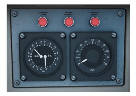
m.r. and b.c. gauge – combined main reservoir and brake cylinder pressure gauge.
