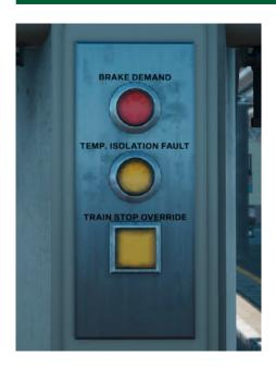
BRAKE DEMAND lamp – illuminates if the safety system activates and indicates that the emergency brakes have been applied.
