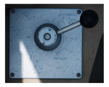
Moving the lever to the rear will release the brakes from EMERGENCY to RELEASE via FULL SERVICE, STEP 2 and STEP 1. The normal position when stopped is FULL SERVICE.
