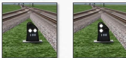
In TSC this signal is used only as a subsidiary signal of the departure signal and placed immediately after it. When the departure signal is " (Blocked Path) for train, but the shunt signal has the 2 vertical lights switched on, then the train can start because is directed to a shunting destination track, not on the main line.
