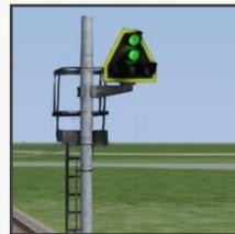
The protection version is indicated by a square black plate with yellow border. If it shows 3 horizontal red lights, means that the protected CL is open. If it shows 2 vertical green light, means the protected CL is closed.
