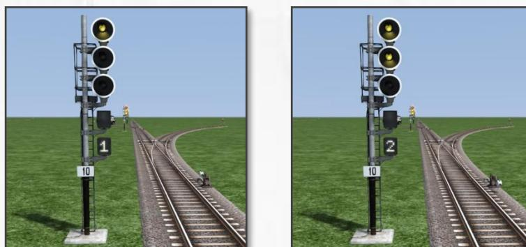
The direction display is always switched off when the signal is in Blocked Path condition (R).
