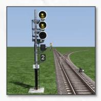
The direction display is always switched off when the signal is in Blocked Path condition (R).
