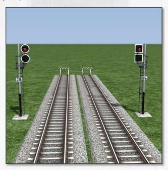
In some stations, in case of multiple parallel tracks, the rule is still the same. Circular shape if placed on left of the track, square shape if placed on the right of the track.
